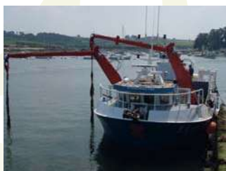
(2) Vessel with a « scoubidou », used to harvest Laminaria digitata on the coasts of Brittany (France) © Maguire.
