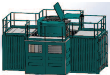
Deployed maritime ISO-20" container, used as a fully integrated digestion station at the end-user site.
